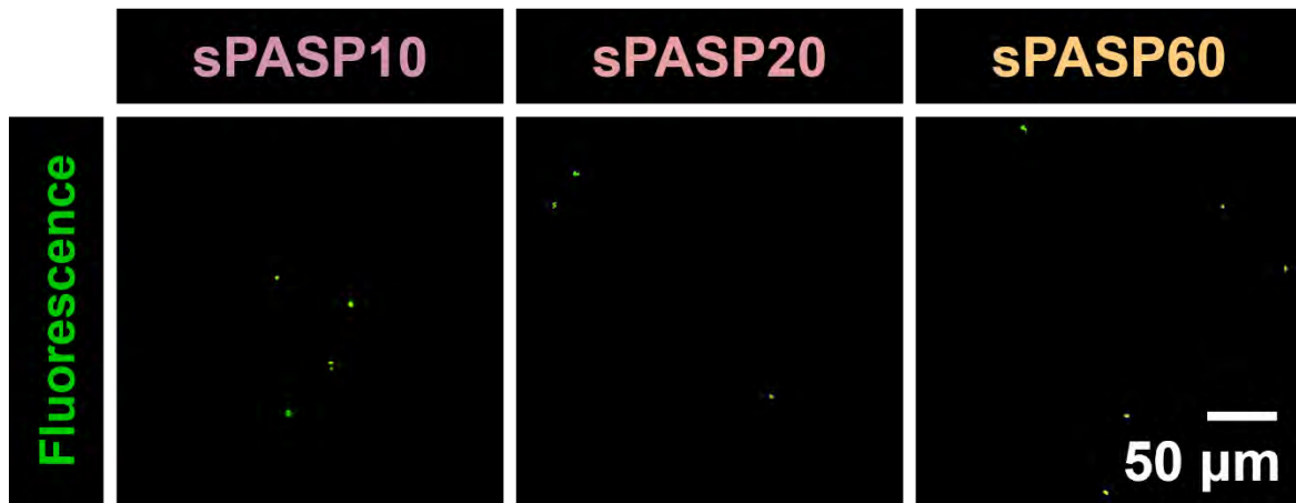
Figure S5. Visualisation of platelet adhesion on sPASP10, sPASP20, and sPASP60 surfaces using fluorescence microscopy.
