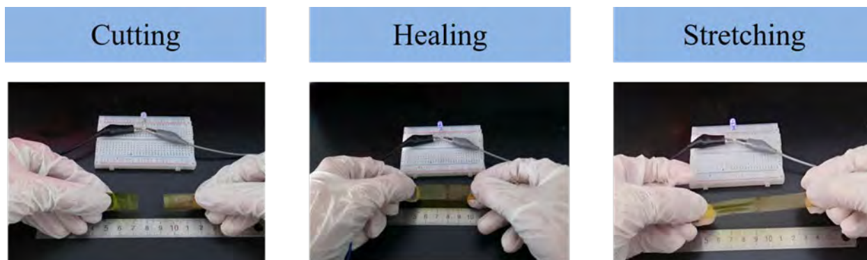
Figure S3. Electrical self-healing behavior of the GCAM7 hydrogel conductor. The sequence shows cutting, self-healing, and subsequent stretching of a damaged hydrogel strip while the LED remains lit, demonstrating restoration of conductivity after healing.
