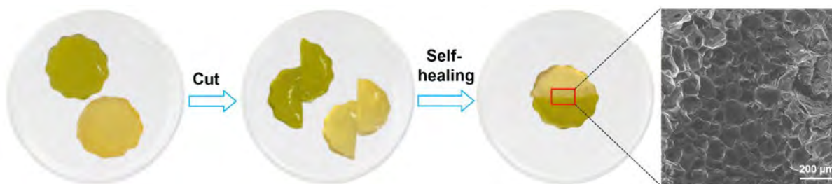
Figure S4. Optical images and SEM micrograph of cut and self-healed specimens, in which the fracture interface disappears, and the porous network becomes continuous, providing visual evidence of the reconstructed microstructure.
